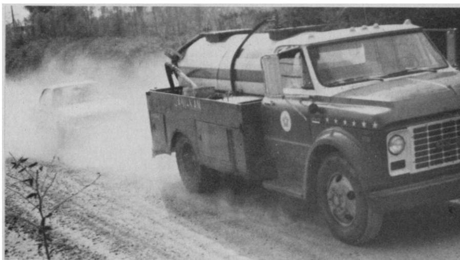
Fig. 1. A cloud of dust follows vehicles traveling on a road surfaced with crushed serpentinite, a large proportion of which consists of fines and small friable rock fragments. Samples of suspended air particulates taken in the vicinity contained a large number of chrysotile asbestos fibers.
