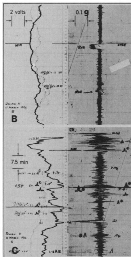
Fig. 2. Dual traces of CAT radiometer output (left) and accelerometer (right). (Top) A situation without CAT with a normal radiometer output ( $C < 0.4$  volt  $\text{sec}^{-2}$ ). (Bottom) Situations characterized by CAT encounters with anomalous radiometer outputs ( $C > 0.5$  volt  $\text{sec}^{-2}$  in all cases); alert times range from 4 to 10 minutes. Altitude, 13.5 km; date of measurements, 11 March 1976.
