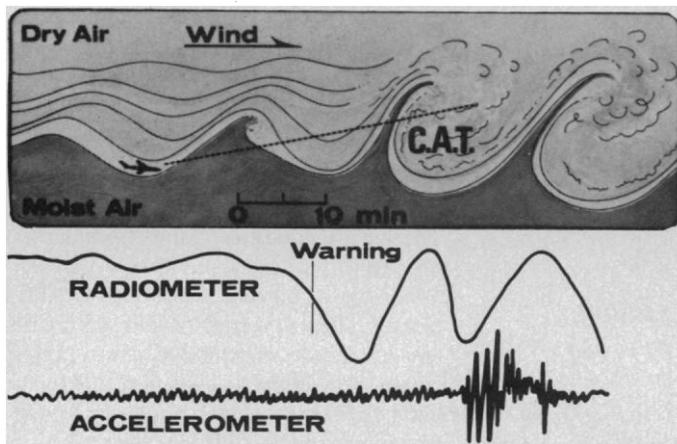
Fig. 1. Schematic showing the C-141A heavy jet in advance of the breaking KH waves. Lines in the lower portion show hypothetical radiometer and accelerometer traces.
