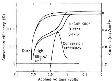
**Fig. 1.** Current-voltage and conversion efficiency-voltage diagrams for a cell made of Zn-doped GaP,  $\langle 111 \rangle$  as the cathode and Pt foil as the anode. The electrolyte was  $10^{-2}M$  NaOH +  $0.5M$   $\text{Na}_2\text{SO}_4$ . The light source was an attenuated, water-filtered, 75-watt Xe lamp.
