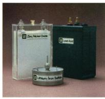
Motors recently has moved more energetic batteries a step closer to reality. Our Electrochemistry Department successfully developed and tested a compact lithium/iron sulfide cell that achieved
