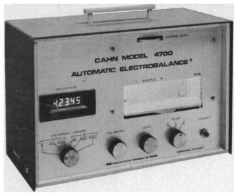
Fast, accurate weighings are automatic on Cahn's new 4700. You simply put your sample on the pan and the balance does the rest. The weight appears automatically on the digital display...with no possibility of operator error...with a readability of 0.1 ug. For complete details and
