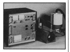
First we designed and produced the 9910 Tube Series for improved images, reduced magnetic field and smaller tube diameter, together with a compact air-cooled focus coil.
