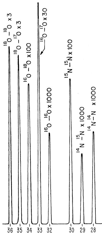
Fig. 4. Mass spectrum of an equimolar mixture of nitrogen and oxygen containing: 28 atom percent  $^{15}\text{N}$ ; 3.3 atom percent  $^{17}\text{O}$ ; and 6.9 atom percent  $^{18}\text{O}$ . [Courtesy Vandervoort and Gomez (61)]
