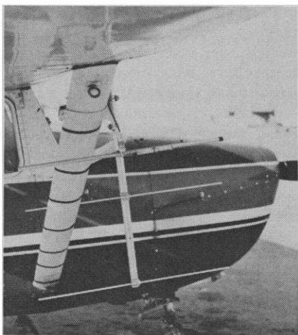
Fig. 1. The 222-Mhz antenna installed on a Cessna 150 airplane.
