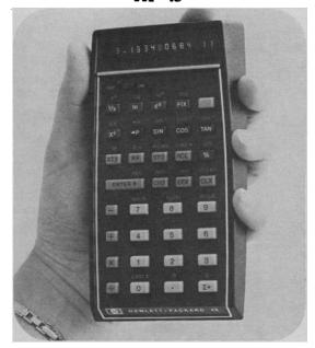
matically stored. You can recall this number by pushing the "Last X" key...then proceed to correct it or to perform calculations with it.
