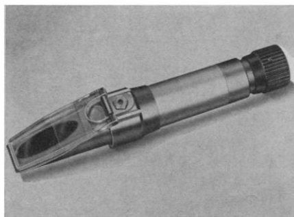
Fig. 1. National Instrument Company's model 6 hand refractometer provides high-contrast reading of concentrations from 0 to 32 percent and reads directly to 0.2 percent.
