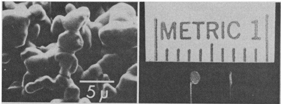
Fig. 1 (left). Scanning electron micrograph of fused tantalum meshwork showing large available surface area (7). Fig. 2 (right). Capacitor electrodes designed for surface stimulation of cerebral cortex.
