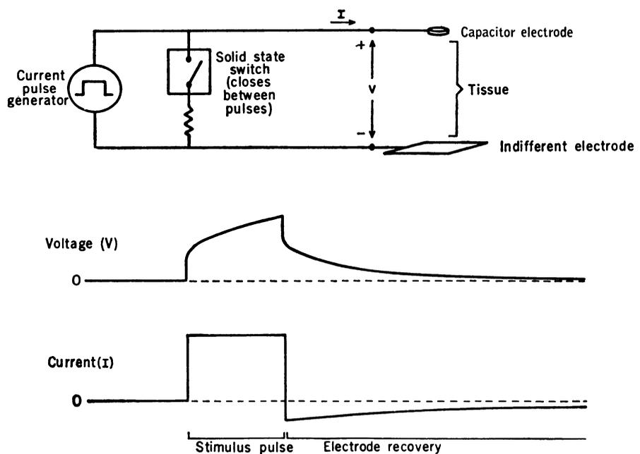
Fig. 3. Typical stimulating circuit with resulting voltage and current waveforms.
