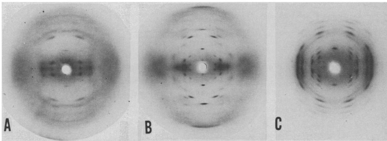
Fig. 1. X-ray diffraction patterns of stretched films of chondroitin 6-sulfate (A and B) and a new (low-humidity) form of hyaluronate (C). We interpret these patterns as arising from (A) threefold helices packed in a trigonal array, (B) eightfold helices in a tetragonal array, and (C) fourfold helices also in a tetragonal array. The direction corresponding to the parallel axes of the helices is vertical in all cases.
