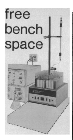
ISCO's miniature fraction collector frees up to 2 or 3 square feet on your lab bench. Newest of the Golden Retriever series, the Model 1200 Pup holds 95 test tubes in removable, self-standing racks of 5 each, yet measures only 9" by 11%"—about the same as this magazine
