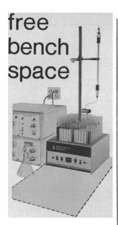
ISCO's miniature fraction collector frees up to 2 or 3 square feet on your lab bench. Newest of the Golden Retriever series, the Model 1200 Pup holds 95 test tubes in removable, self-standing racks of 5 each, yet measures only 9" by 11¼"—about the same as this magazine
