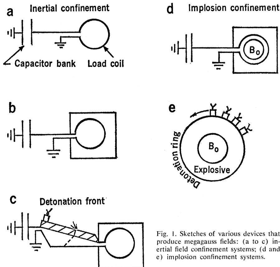
Fig. 1. Sketches of various devices that produce megagauss fields: (a to c) inertial field confinement systems; (d and e) implosion confinement systems.
