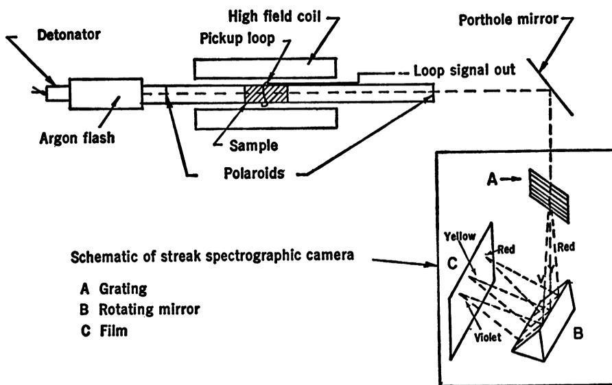
Fig. 3. Schematic drawing of the system used for megagauss field optical experiments. Light passing through the sample is directed to the spectrographic sweep camera which splits the light by wavelength and focuses it on the film at a position determined by the orientation of the rotating mirror.
