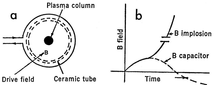
Fig. 2. (a) End view of a  $\theta$ -pinch device that produces high-temperature plasmas. (b) Magnetic drive fields as produced by a capacitor bank and by implosion.
