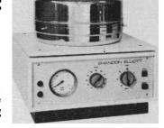
synovial fluid, peritoneal exudates, seminal or other body fluids. Centrifugation and slide preparation are performed simultaneously, which eliminates prior centrifugation and saves you time. Improved head design ensures safety when working with pathogenic organisms.
