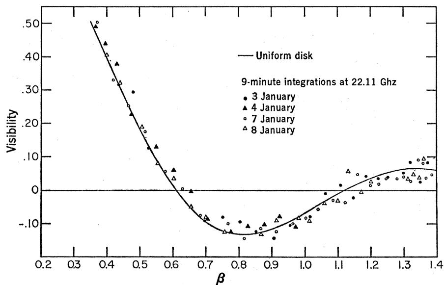
Fig. 2. Visibility function of Venus. The quantity  $\beta$  describes the interferometer fringe cycles per disk radius, and is proportional to the baseline projected in the direction of the source. The data points show 9-minute averages obtained during 4 days in January 1971. The visibility function which would be produced by a uniformly bright disk of the radius of Venus is drawn for reference.
