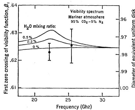
Fig. 3. Limb darkening resonance of Venus. The measured first zero crossing of the visibility function is a measure of the overall limb darkening of the apparent disk. The addition of water to the atmosphere would produce additional, frequency-dependent limb darkening due to the 1.35-cm rotational transition, as shown by the solid curves. The two data points represent 8 days of averaging at 22.11 Ghz and 4 days at 25.4 Ghz. (Error bars, 1 S.D.)
