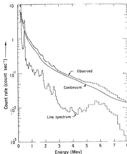
Fig. 1. Apollo 16 pulse-height spectrum, 270-minute accumulation, over 1° to 73°W. (Upper curve) Transmitted data; (middle curve) featureless continuum; (lower curve) net line spectrum.
