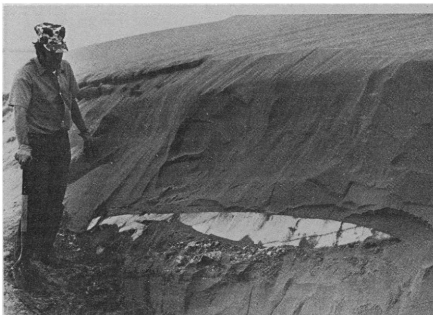
Fig. 1. One of several snow lenses still preserved in eolian dune sand 4 months after the last snowfall. The lens is 25 cm thick, 2.5 m wide, and 1.5 m beneath the surface.
