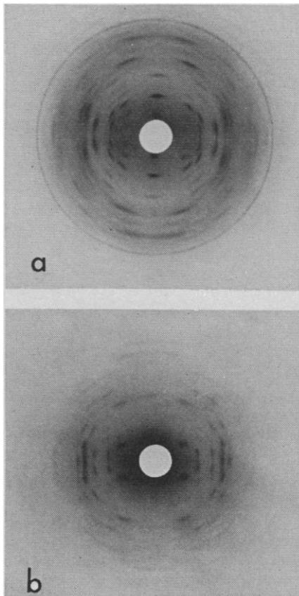
Fig. 1. X-ray diffraction photographs obtained from two new crystalline forms of potassium hyaluronate. Similar patterns were also obtained for sodium hyaluronate. The pattern in (a) is interpreted in terms of a double-strand helix (3), and that in (b) in terms of an untwisted version. The fiber axis is approximately vertical in each case.
