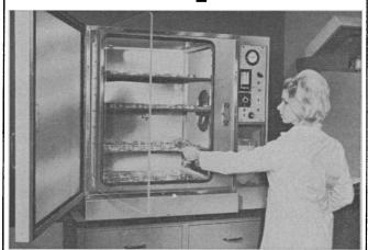
Designed to meet the most stringent research requirements, this new  $\mathrm{CO}_2$  incubator provides a carefully controlled, high humidity  $\mathrm{CO}_2$  environment. The unit has a 7-1/2 cubic foot working chamber, yet needs little bench space. Temperature is electronically controlled from ambient to 70°C, and  $\mathrm{CO}_2$  tension is maintained from ambient to 20%. Other features include an automatic  $\mathrm{CO}_2$  recovery system and a visible water reservoir.
