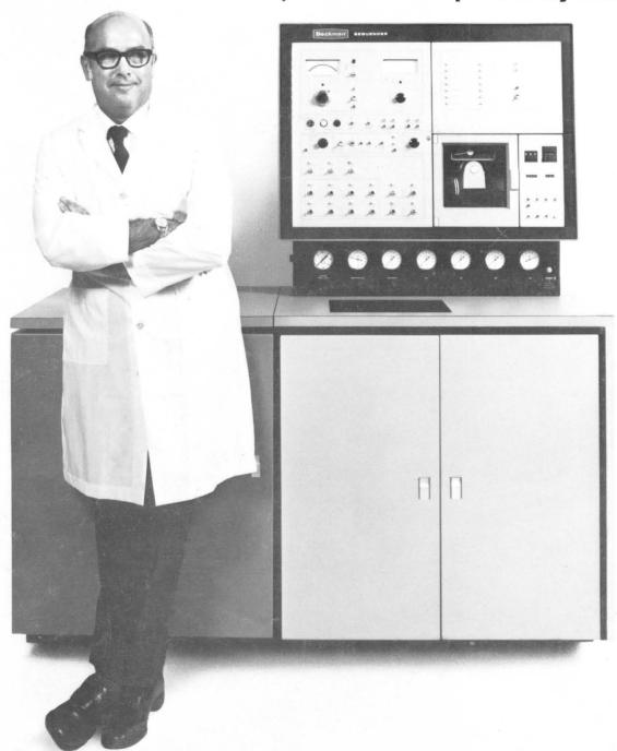
Sequencing proteins can be done very rapidly indeed with the help of a Beckman 890C Automatic Sequencer. One residue per hour -24 a day.
