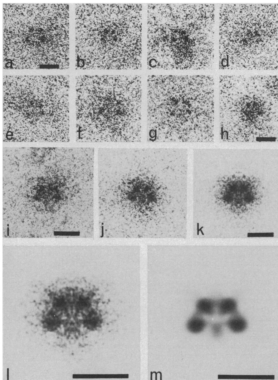
Fig. 1. (a to h) Dark field electron micrographs of eight individual molecules of 2,3,4,5-tetraacetoxymercurithiophene. (i to k) Visually aligned photographic superposition of (i) 4 molecular images, (j) 16 images, and (k) 64 images (32 individual molecules plus a reflection). (l) Computer assisted superposition of 64 images. (m) Image in (l) optically filtered to a resolution corresponding to 2.6 Å. (a to m) The scale is 10 Å.
