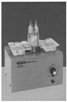
Bagless desalting with Bio-Fiber® hollow fiber devices is rapidly replacing conventional methods. Why? Because it's so quick and simple (95% salt free in 20 min.). Equipment needs are simple too. For best results you require:
