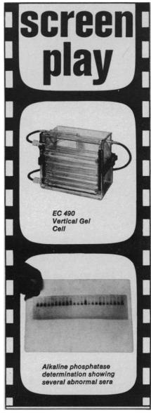
Screening protein mixtures for analytical or preparative work isn't tedious when you use an EC 490 Vertical Gel Cell. This simple, easy-to-operate unit handles up to 30 samples at one time. Using only one convenient polyacrylamide gel slab means uniform conditions for all samples, uniform comparison.
