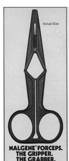
You get a powerful grip on tiniest, tissue-thin objects . . . a positive clamp on vinyl or rubber tubing. Use with hot or corrosive materials. May be autoclaved or gas-sterilized for re-use, yet low enough in cost to be disposable. This is the unique multi-purpose, all-plastic Nalgene forceps . . . remarkably efficient and inexpensive.
