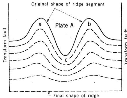
Fig. 4. The effect of surface cooling in the development of an orthogonal ridge transform fault pattern.
