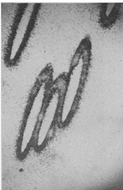
Fig. 7. Micrograph of the uranium distribution in taper-sectioned wires (0.005 centimeter wide) with uranium-enriched tin diffused into a thick outer section of the niobium wire to produce a layer of \text{Nb}_3\text{Sn} . Induced uranium fission tracks clearly delineate the thickness of the uranium-rich layer, which is the same as that of the \text{Nb}_3\text{Sn} sheet.
