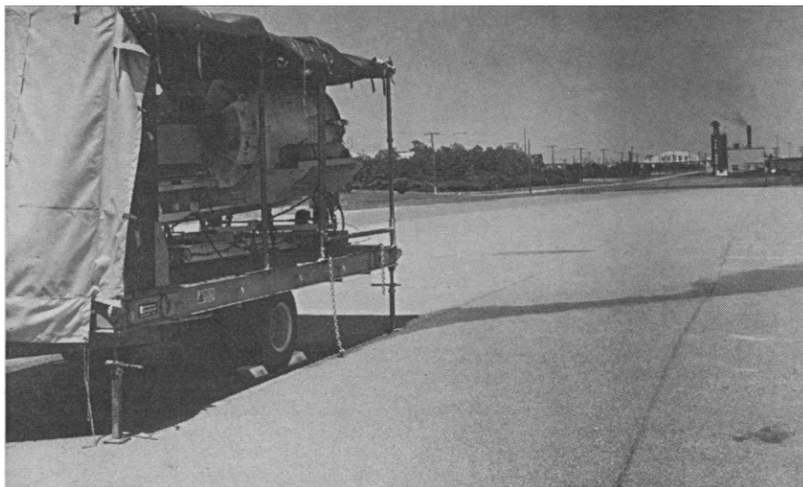
Fig. 1. Monitoring emissions from a distant smokestack with Block Engineering's remote laser Raman spectrometer.
