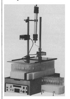
Effluent peaks between recorded event marks aren't always deposited in the indicated test tube. Event marks locate tube changes, but the adjacent curve monitors the effluent as it is passing through the flow cell, not into the tubes. The resulting discrepancy can be quite large if the effluent tubing, flow rate, and collected sample size are not perfect. Manual chart corrections are inaccurate and time consuming.
