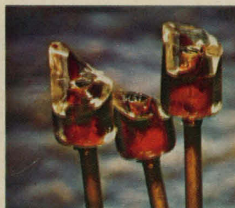
Macro photograph, diode fractures
