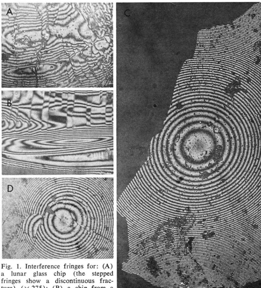
Fig. 1. Interference fringes for: (A) a lunar glass chip (the stepped fringes show a discontinuous fracture) ( $\times 275$ ); (B) a chip from a piece of industrial glass showing multiple cracking ( $\times 275$ ); (C) a lunar glass chip with a concave spherical surface ( $\times 165$ ); and (D) a lunar spherule with pieces chipped off ( $\times 220$ ).
