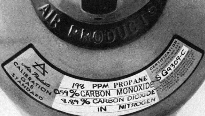
When you work with certified calibration gases, you want to know the exact analysis in the cylinder you're using. No matter whose gas it is, one cylinder's composition can differ from the next by a fraction of a percentage point.
