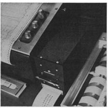
Digital printout simplifies electrophoresis. Electrophoresis densitometer
