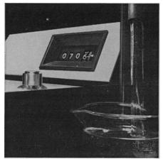
pH meters with digital readout give faster, more accurate readings regardless of operator fatigue.
