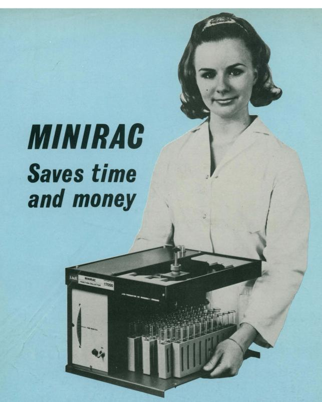
You can save time and money by using the MiniRac for all the less-complicated fraction collecting in your laboratory. It does these jobs just as well as more sophisticated and costly instruments. Up to 60 fractions can be collected, automatically, in one run and dispensing time per fraction can be set for 1 to 40 minutes. An event-marking outlet is incorporated, making the MiniRac suitable
