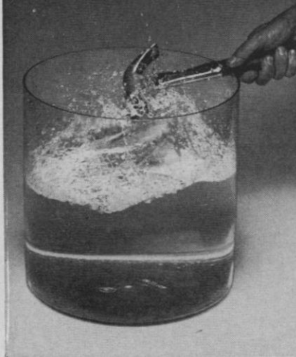
Here are the unbreakable, economical successors to standard-size glass cylindrical jars. You can safely drill, tap, or apply clamps. Heat resistant to 135°C. Use them as water baths, terraria, aquaria, bell jars, environmental chambers, for freeze-drying and other vacuum applications, and as large transparent, autoclavable containers.
