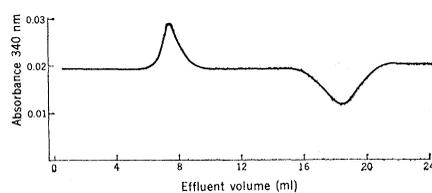
Fig. 1. Elution of LADH-NADH complex ( $3.1 \times 10^{-6}N$ ) from a Sephadex G-50 column ( $1.0 \times 26$  cm) equilibrated with NADH in 20 mM phosphate, pH 7.0 at 25°C.
