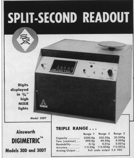
When you place a sample of unknown weight on the pan of this top loading balance, the correct answer is shown *instantly* on a 5-digit readout. There are no weights to dial, no problems with parallax and overhead glare, no spring hysteresis.
