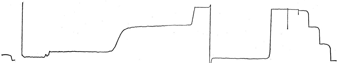
Fig. 1. Sedimentation velocity of reconstituted incubation mixture at pH 7.0 and 19.3°C. The photoelectric scanner pattern was taken at 280 nm 40 minutes after a speed of 30,000 rev/min was attained.
