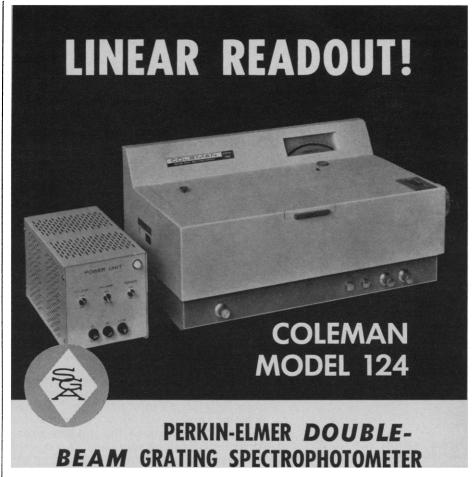
This instrument is the only one in its class offering meter readout that's linear in both transmittance and absorbance. It provides fully automatic ratio-recording; gives you the capabilities of both a double-beam automatic and a single-beam manual spectrophotometer; and, now that eight major accessories are available, Model 124 is even more versatile than before.
