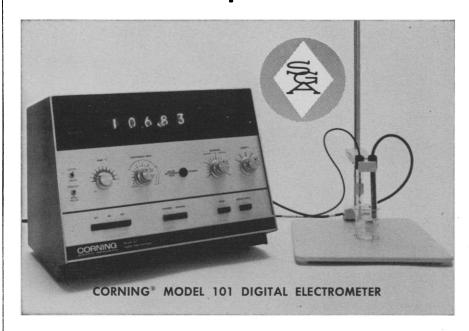
For the first time — direct digital readout of ionic activities or concentrations ... in moles per liter, milliequivalents per liter, parts per million (or others).
