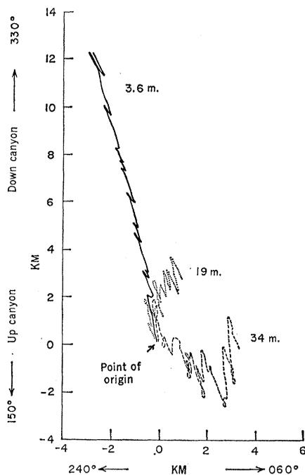
Fig. 2. Trajectories of the movement of particles of water at three depths above the floor of La Jolla Canyon where the axis is 206 m deep.
