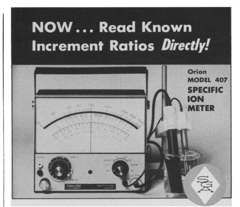
Not only can you use this portable instrument with all specific ion electrodes, with all pH electrodes, and with all redox electrodes, but thanks to a special meter scale, it is now possible—for the very first time—to read known increment ratios directly! You don't have to know the composition of the sample, nor prepare background solutions. All you have to do is measure out the sample, add a known amount of the ion being measured, and read the ratio directly on the scale.
