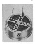
Insulated double-walled bath rotates on a fixed base permitting free access to all tubes. Removable two-tier support retains tubes with pipettes in an upright position, with or without ice in bath.
