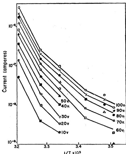
Fig. 2. Current as a function of reciprocal temperature for different voltages.
