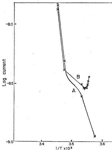
Fig. 3. Log current as a function of reciprocal temperature at 1 volt in the dark (curve A) and under illumination by 5 mw of light from 4200 to 5000 Å (curve B).
