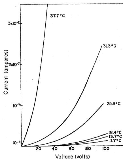
Fig. 1. Current as a function of voltage at different temperatures for a sample 0.8 by 0.8 by 0.5 cm thick.
