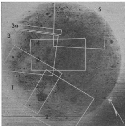
Fig. 1. Infrared image of the eclipsed moon reconstructed from 200 line scans recorded during the eclipse of 19 December 1964. Black areas are warm. The areas scanned during the 13 April 1968 eclipse are outlined. (Infrared image from Shorthill and Saari, 1965.)
