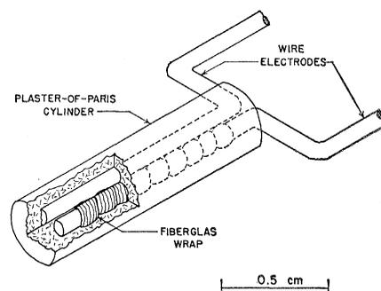
Fig. 1. Diagram of the moisture-tension sensor for plants.
