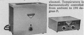
**3. Blackstone U-20 Cell Disrupter.** A highly flexible unit designed for routine continuous or batch processing of cell suspensions, chemicals and solutions common to research in biochemistry, cytology, microbiology and related fields. Laboratory tests show that employing a 70 ml. volume of a 20% suspension of Escherichia coli, 98% disruption was achieved in 12 minutes with no loss of activity in enzyme Beta Galactosidase. 0 to 100% power control for complete processing flexibility.
