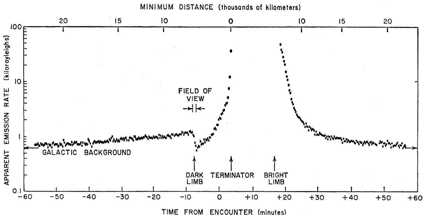
Fig. 1. Signal obtained from the lithium fluoride-Lyman alpha channel during the Venus encounter. Times when the photometer observed the dark limb, terminator, and bright limb are indicated. The minimum-distance scale gives the perpendicular distance from the photometer line of sight to the center of the planet.
