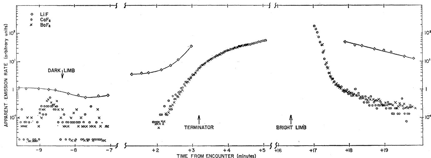
Fig. 2. Signals obtained from the three photometer channels during critical periods of the Venus encounter. Three expanded time intervals are shown: dark limb, terminator, and bright limb.
