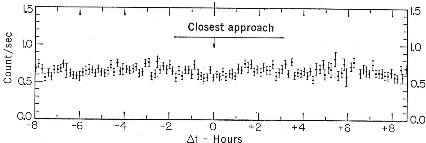
Fig. 1. Counting rate of the electron detector ( $E_e > 45$  kev). Each point represents the average counting rate for a 216-second sampling period. Error bars show the statistical standard error of each point. The lowest daily average rate of this detector which has been observed during its flight to Venus is  $0.59 \pm 0.01$  count/sec (due primarily to galactic cosmic rays).
