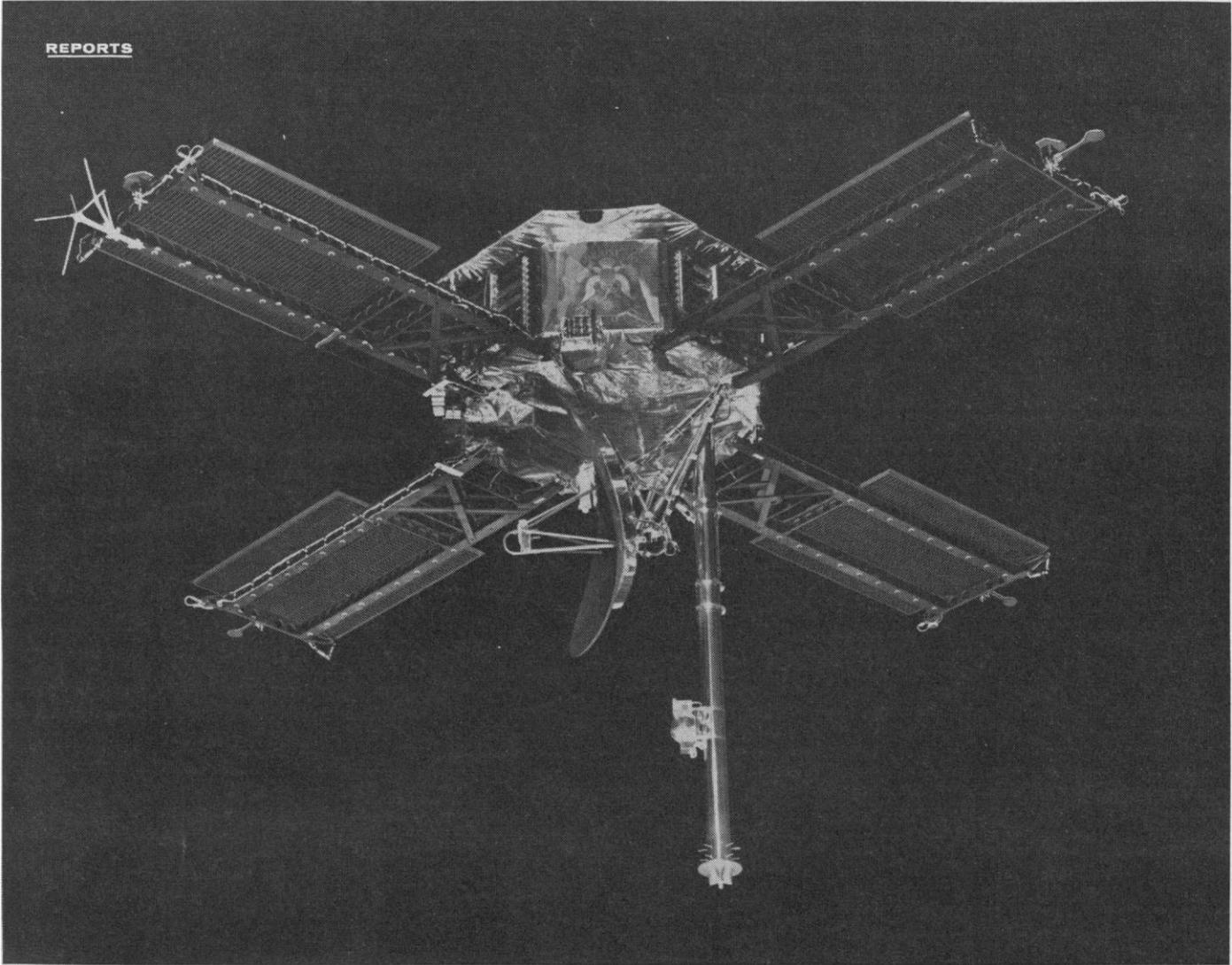
Fig. 1. The Mariner V spacecraft as it would have appeared if visible from Earth about 60 days after launch. Its top side, facing Sun, is almost flat except for the plasma sensor and solar attitude sensors. The bottom side carries several of the scientific instruments as well as the parabolic directional antenna and the mast-like "omnidirectional" antenna, on which the magnetometer is mounted. The receiving antenna for the 423-Mhz signal extends from the tip of the solar panel at the upper left.
