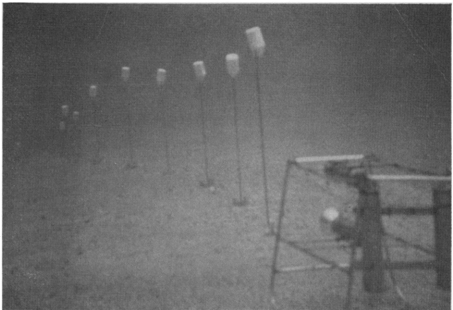
Fig. 1. A camera and a line of targets, 4-liter bottles spaced 3 m apart, photographed at a depth of 183 m under ambient light; the depth of field exceeds 30 m.
